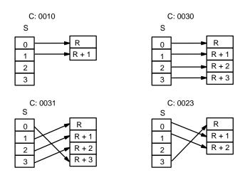
The following is an example of a one-digit decode operation from digit number 1 of S, i.e., here C would be 0001.
